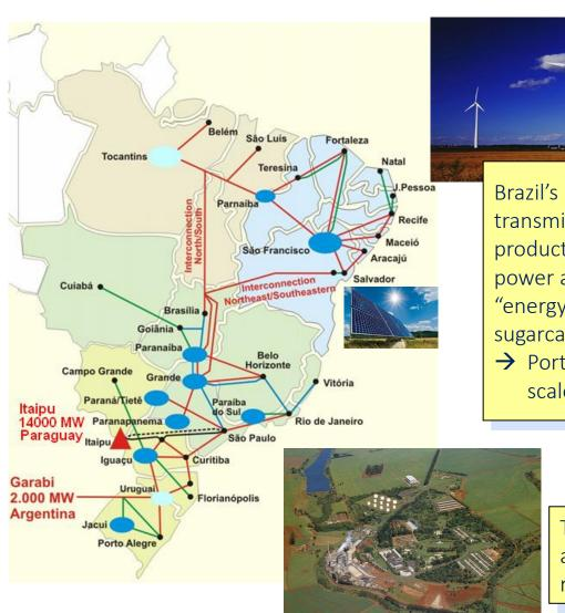
Brazil's hydro reservoirs and the countrywide transmission grid are used to modulate the seasonal production of biomass and the fluctuations of wind power and solar; the system reservoirs are used as "energy warehouses" that may "store" wind, sun and sugarcane
